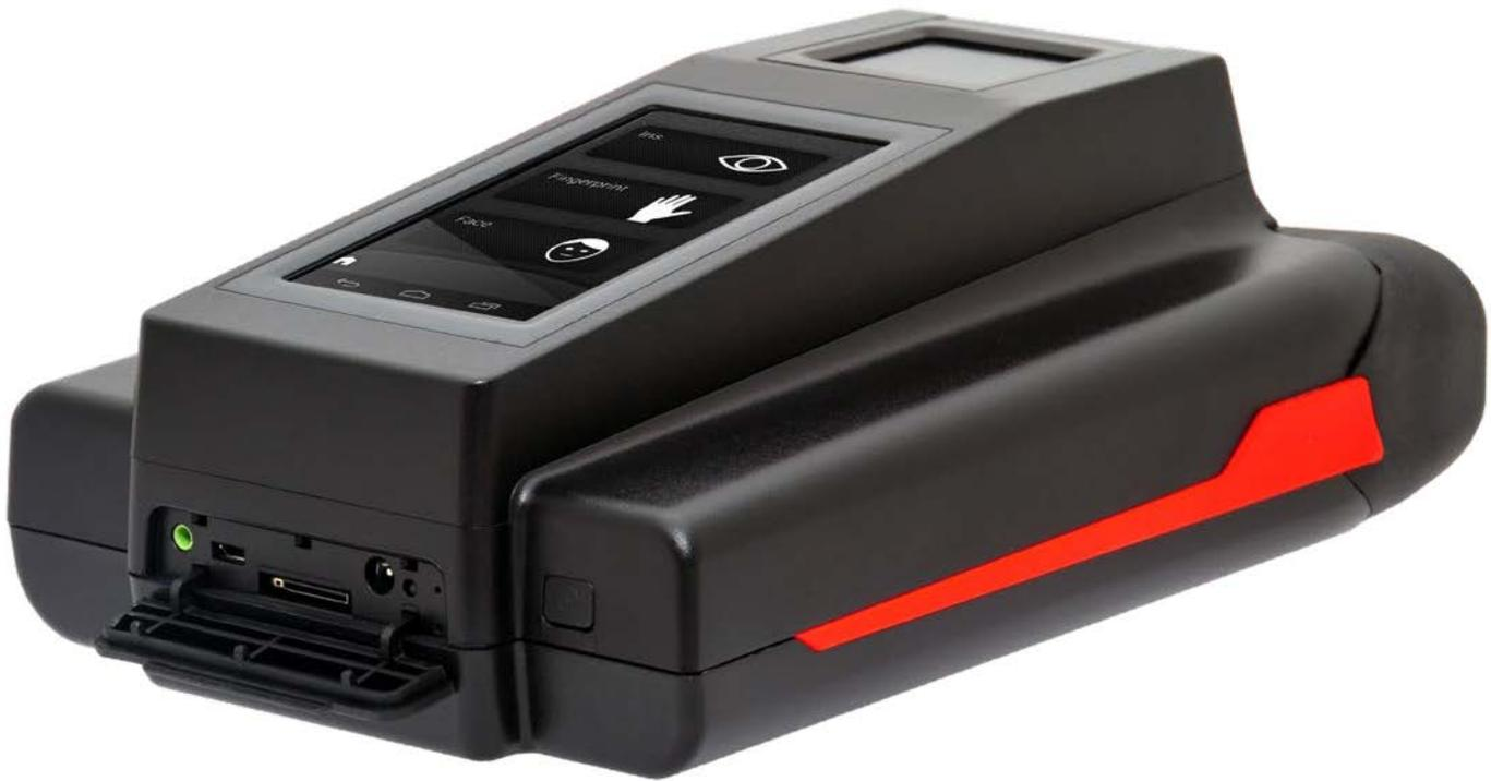
**Trident** is a completely integrated multi-modal mobile biometrics device that employs the world's smallest and fastest FAP 45 fingerprint scanner, the first binocular-type iris capture on a mobile device and a stunning 5 MP auto-focus camera with flash.
